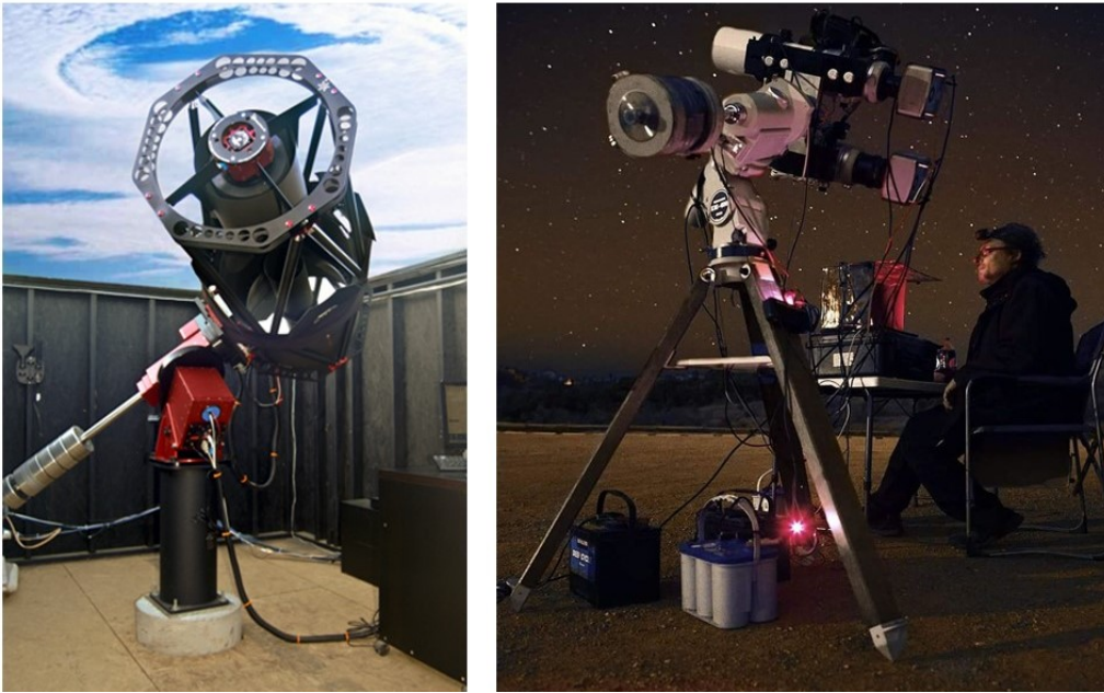
Figure 1. Two examples of the amateur equipment used in ultra-deep imaging of nearby galaxies shown in this review: ( Left ): The Officina Stellare PRO RC 500 half-meter telescope from the Black Bird II Observatory, located at 1,410 meters elevation in the California Sierra-Nevada Mountains near Alder Springs, California. ( Right ): Portable equipment composed by a double Takahashi FSQ106EDX, each one with a CCD camera SBIG STK11k CCDs. (Image credits: R.J. Gabany & R. Bernal)
